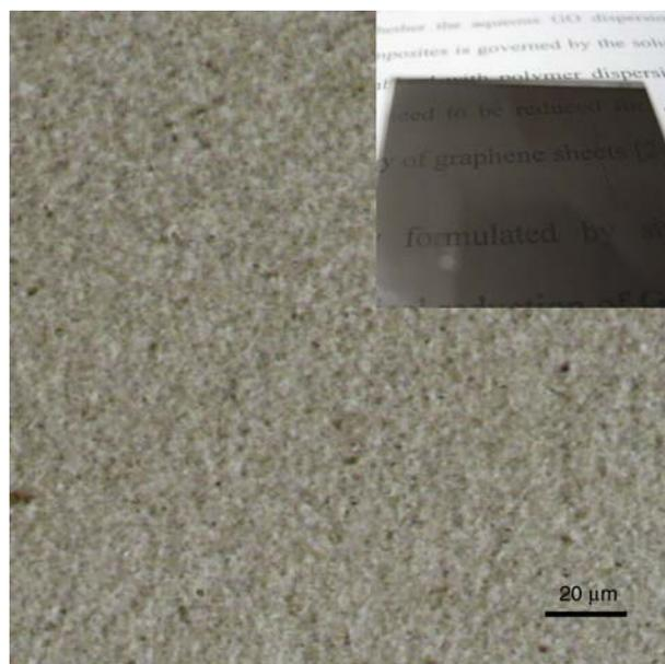
**Figure 7.** Optical microscopy images of uncured epoxy containing 0.26 vol% fGO coated on glass substrate. Inset shows a picture of the dispersion between glass slides
