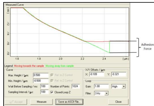
Figure 4: Adhesion force in force-distance curve from PHM50
