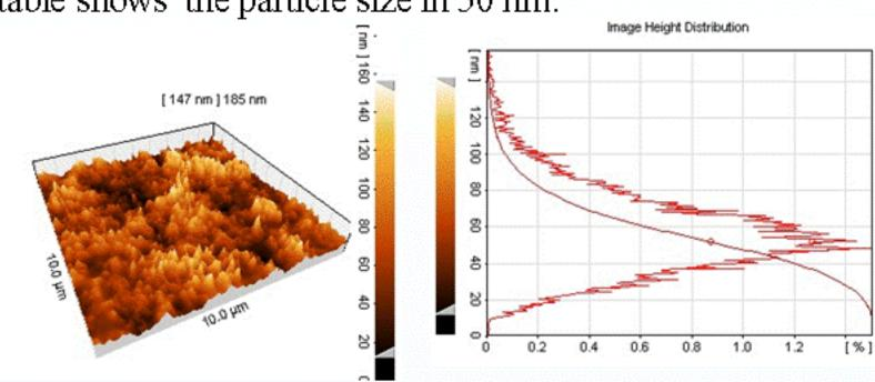
Because the viscosity of the MEG is high, particle size distribution is so homogeneous and about 3nm
