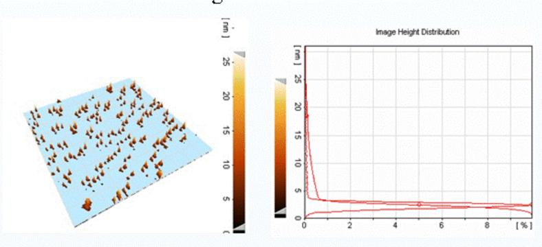
The atomic force microscope image shows octagonal structure for nanosilver. The particle size distribution is about 10nm. Because the solvent is polar.
