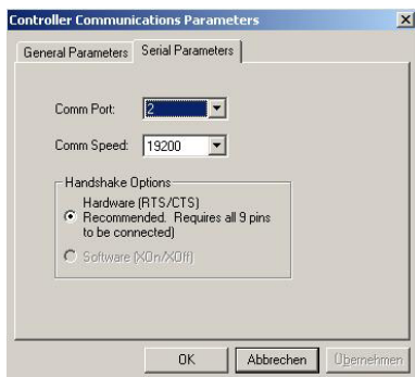
Fig. 36: Setup for GALIL motion controller
