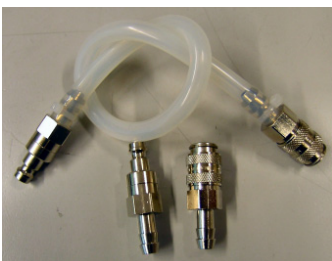
Fig. 4: Bypass tube with mounted quick couplings and quick couplings for mounting the circulator bath
