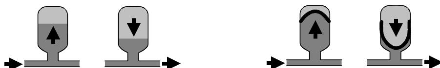
In the case of **pulsation dampers with a separating diaphragm**, the air or nitrogen cushion is separated from the dosing medium by an elastic diaphragm. As a result the cushion cannot dissolve in the dosing medium. Furthermore the cushion can be preloaded, making it also suitable for high pressures.
