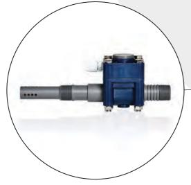
**Injector with safe vacuum technology** The injector for chlorine gas DULCO®Vaq generates a constant vacuum, even at high operating pressures. An integrated non-return valve also prevents water from getting into the vacuum line and thereby guarantees long-term safe operation.
