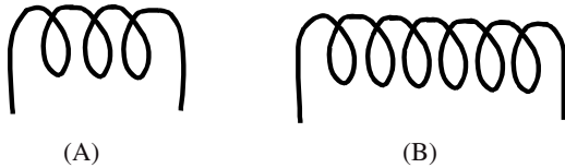
FIGURE 6.80 (A) Few turns, low inductance; (B) more turns, higher inductance. (From Spellman, F.R. and Drinan, J., Electricity , Technomic Publ., Lancaster, PA, 2001.)
