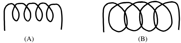
FIGURE 6.82 (A) Small diameter, low inductance; (B) larger diameter, higher inductance. (From Spellman, F.R. and Drinan, J., Electricity , Technomic Publ., Lancaster, PA, 2001.)
