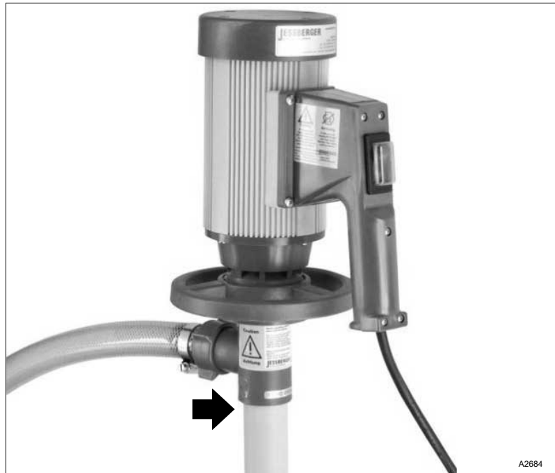
Fig. 6: Lip (arrow) of the outlet nozzle.
