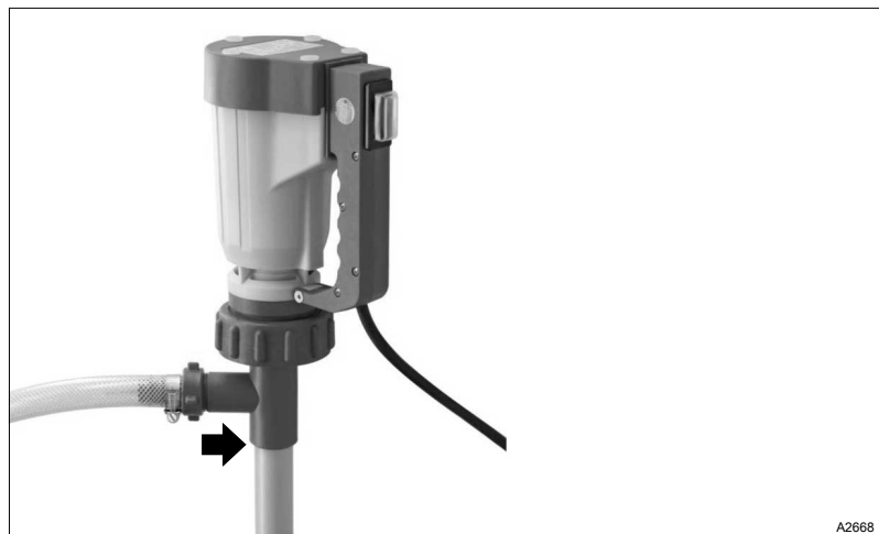
Fig. 6: Lip (arrow) of the outlet nozzle.
