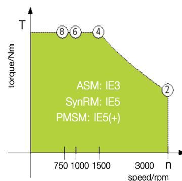
**IE5-permanentmagnet synchronous machines and IE5-synchronous reluctance machines are available with external frequency inverters or as compact drives**
