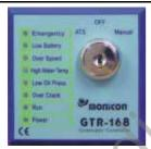
The Model GTR-168is a Manual Engine Control Module designed to control the engine via a key switch and pushbuttons on the front panel. The module is used to start and stop the engine and indicate fault conditions, automatically shutting down the engine and indicating the engine failure by LED, giving true, first up fault annunciation.
